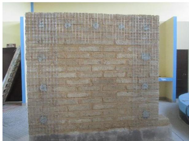
**Figura 17.** Malla electrosoldada instalada
