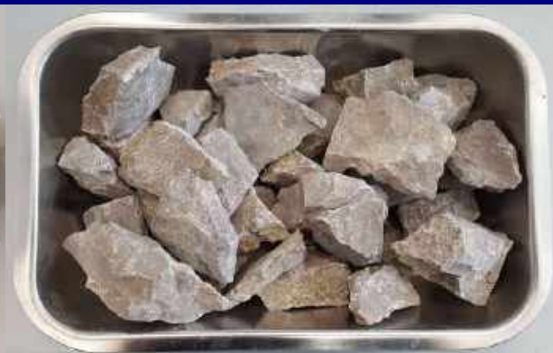
Fig.2 - Carbonate rock sample after crushing
