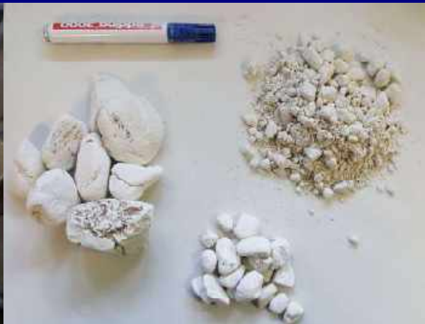
Fig.4 - Lime sample after the degradation test
