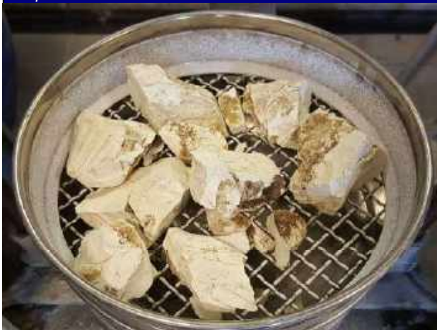
Fig.3 - Lime sample burnt at 1050°C for 3h
