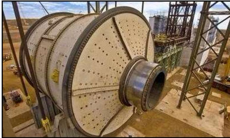
Figura 6: Molino autógeno (Luoyang Zhongtai Industries Co., Ltd., 2015)
