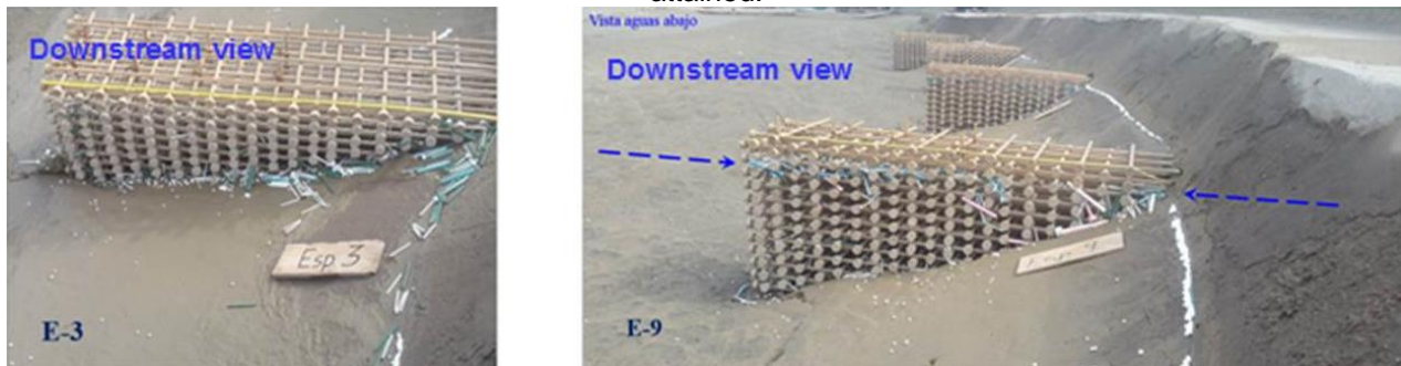
Figure 9. View of groynes E-3 and E-9 in the downstream direction. Notice dowels trapped in the upstream face of the groynes.
